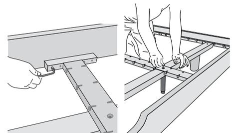
4. Place the bed on its feet. Insert the center rail (6) and fix it with screws. Mount the adjustable center support feet (2) to the center rail (6) using countersunk screws (M8).
