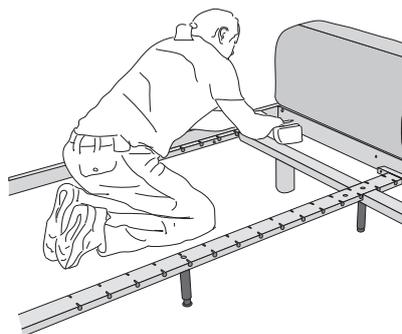
6. Fix the cushions using flat head screws (M6).
