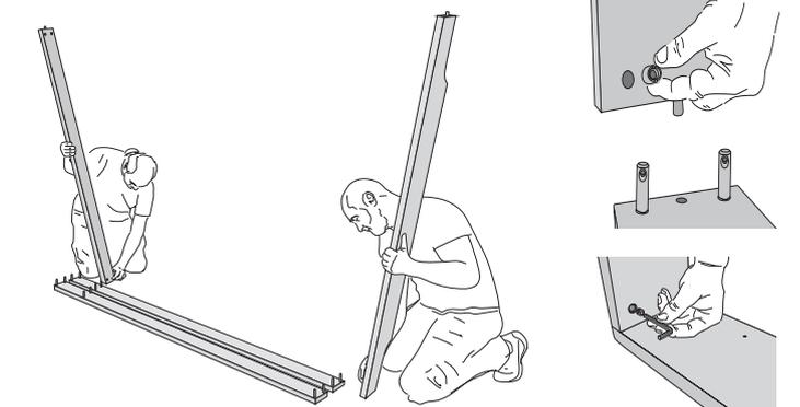
1. Screw XS dowels into side rails (3) and insert the connector housings into the foot and head sections (4) and crossbars (1). Align dowels and housings correctly! Mount foot and headboard (4) as well as the upholstery bar (5) to the side rails and fix with grub screws.
