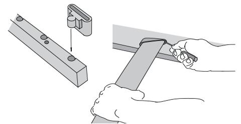
7. Insert the rubber caps into the holes in the mattress supports and fit the sprung slats into the rubber caps.
