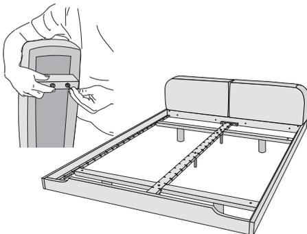
5. Attach the mounting blocks to the bottom of the cushion with the cylinder head screws. Insert the cushions between the head rails (4, 5) the soft side of the cushion facing towards the front.
