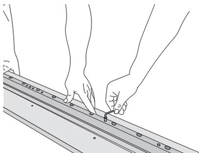
2. Mount the support bars (6) to the side rails (3) using confirmat screws. Screw in the remaining XS dowels.
